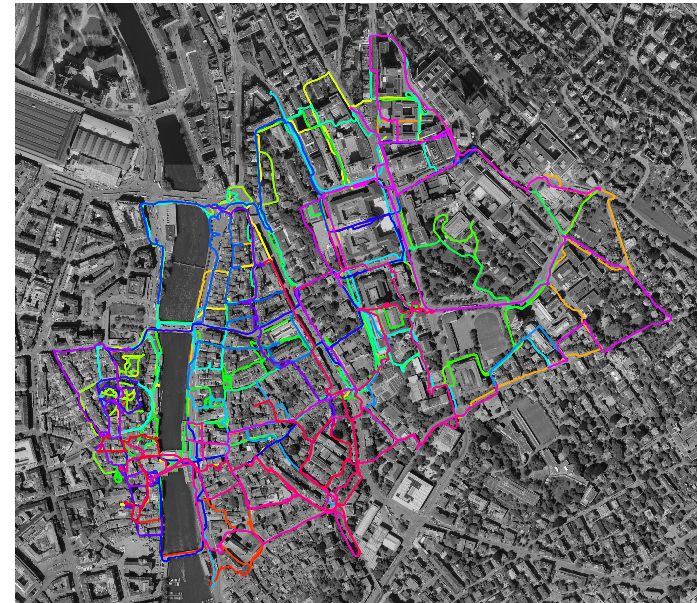
centimetre-accurate ground truth using GNSS/RTK surveyed control points
