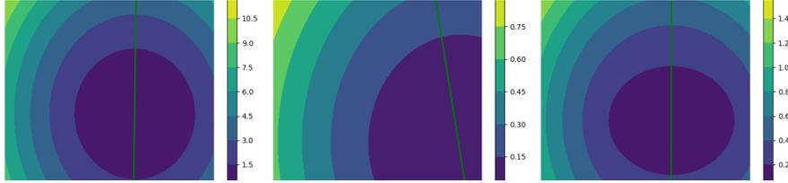
**Fig. 1:** Visualization of the uncertainty of reprojection error for 3D lines at different measured locations. Different from points, the uncertainty of the line reprojection error (point-to-line distance) depends on where it is measured.
